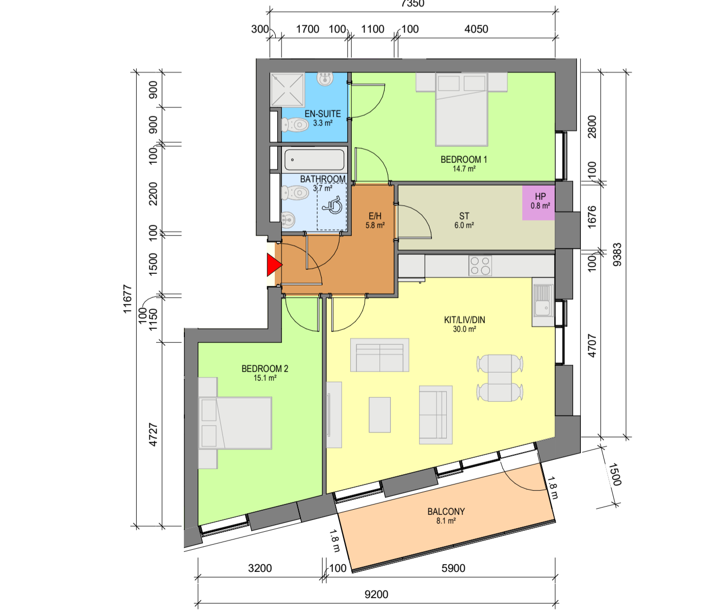
12 Apartment Type 2AJ 1 : 100 - 2 BED, 4 PERSON APARTMENT - NET INTERNAL AREA (NIA) Areas shown in plan - GROSS INTERNAL AREA (GIA) : 83.09sqm
