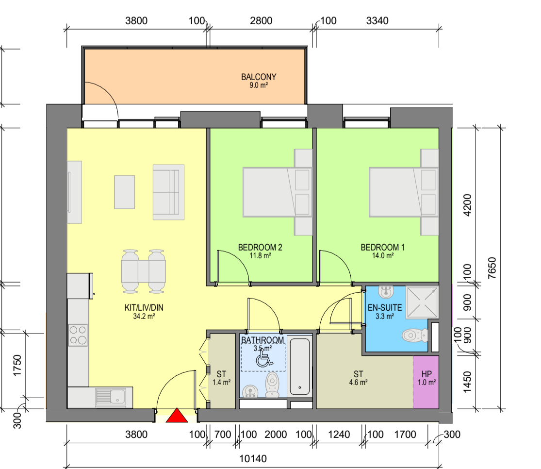
10 Apartment Type 2AH 1 : 100 - 2 BED, 4 PERSON APARTMENT - NET INTERNAL AREA (NIA) Areas shown in plan - GROSS INTERNAL AREA (GIA) : 77.57sqm
