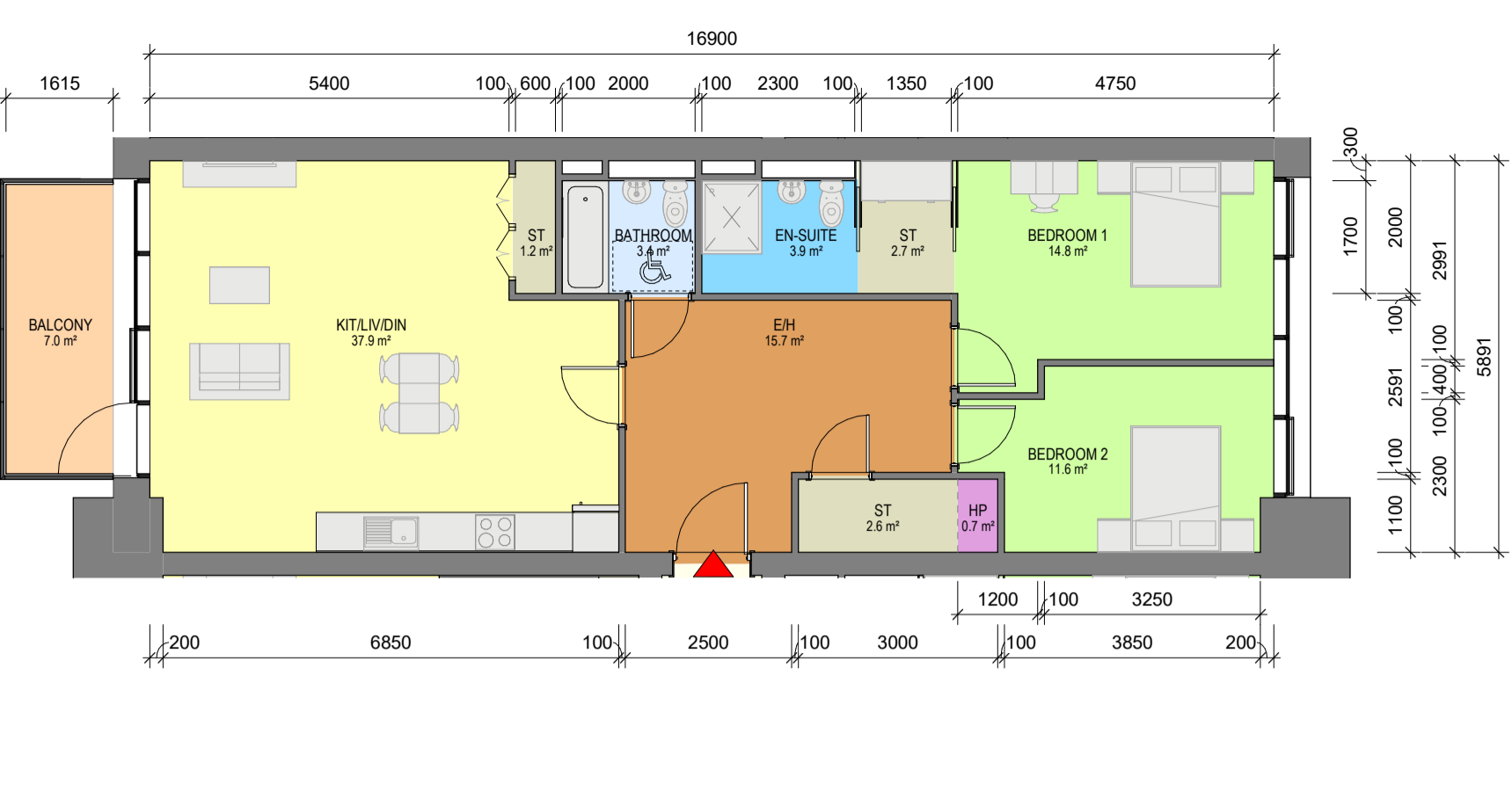
1 Apartment Type 2Y 1 : 100 - 2 BED, 4 PERSON APARTMENT - NET INTERNAL AREA (NIA) Areas shown in plan - GROSS INTERNAL AREA (GIA) : 99.23sqm
